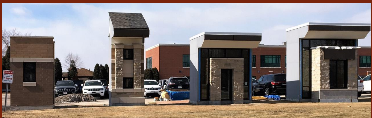
Advanced mock-ups were built to enable testing and simulation of air infiltration levels in the building envelope. In other words, how much air from the inside gets out and vice versa. The mock-ups were built by the contractors using the exact construction materials and finishes for the municipal complex. An independent consultant tested the mockups. Any issues were addressed with the contractors and changes made prior to the actual construction saving both time and money.
