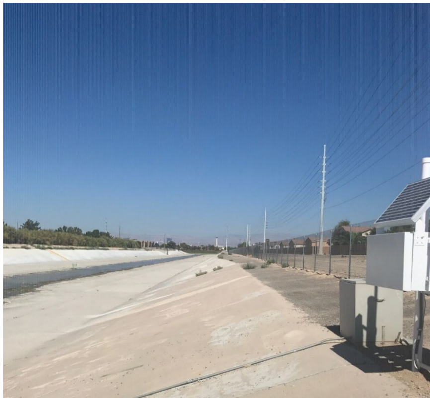
Figure 2-3. Rain gauge and sampler storage box at Club at Sunrise monitoring station
