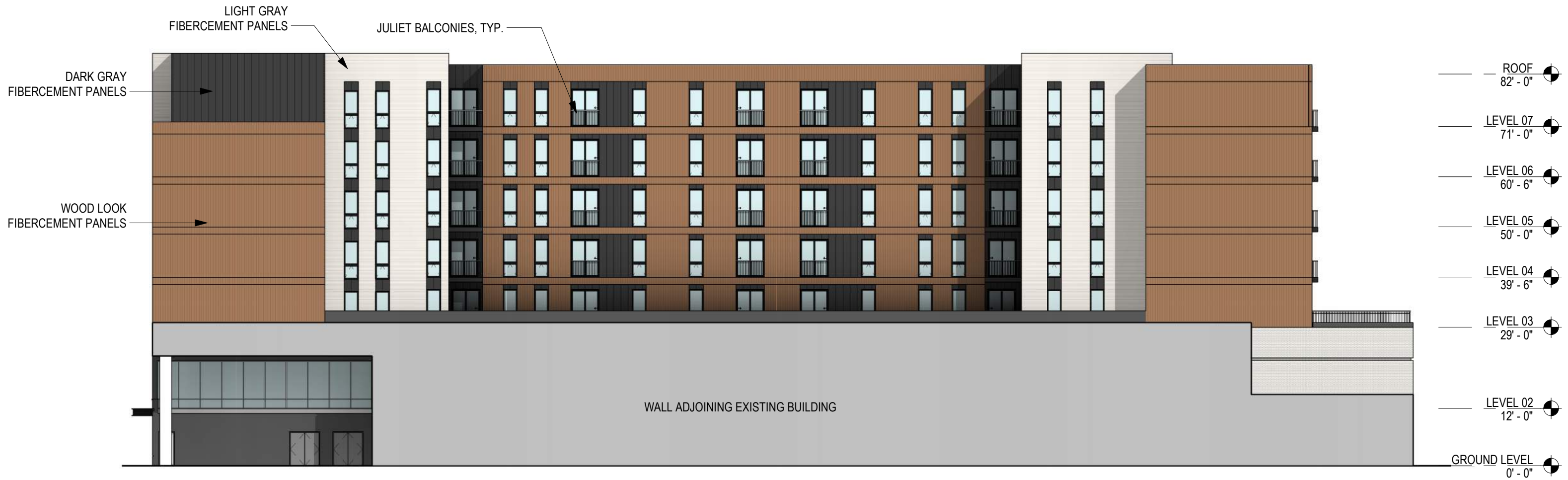
1 11 200_BUILDING ELEVATION_EAST SCALE: 1" = 20'-0"
