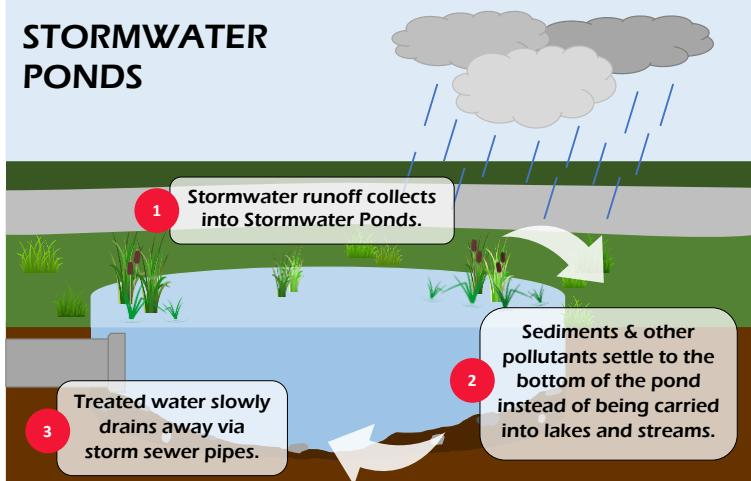
Stormwater Ponds are essential for flood control and water quality. Buildings and pavement cause more rain and snowmelt to run off the land surface rather than soak in, picking up pollutants along the way. The native plants growing along the shore of the ponds, which may look like weeds, are also a benefit to the pond. They prevent shoreline erosion, slow down the flow of stormwater, filter polluted runoff, and provide habitats for fish and other animals.
