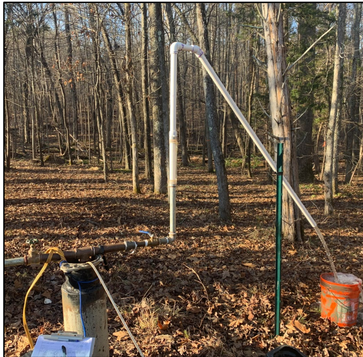
Well AME-X4B Inline Flow Meter and Pumping Test Set up
