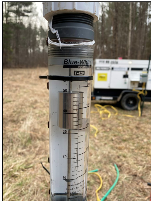
Well AME-X4A Inline Flow Meter and Pumping Test Set up
