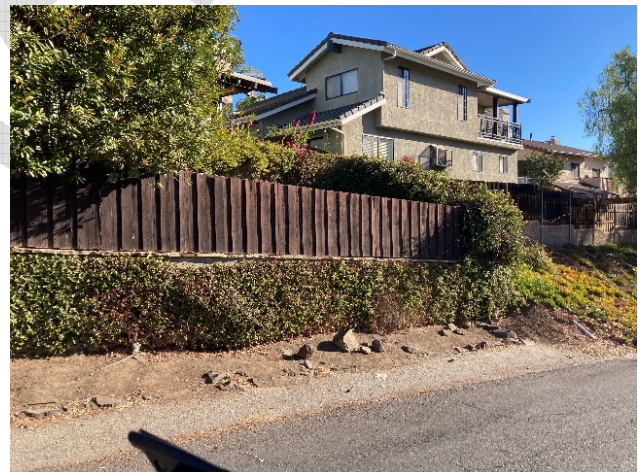
Figure 49: Wooden fences and vegetation near and between homes can act as a "wick" that contributes to fire spread.
