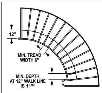
\*Supplement to 2000 IRC Stair Building Code states, "Circular stairways shall have a tread depth at a point not more than 12 inches (305 mm) from the side where the treads are narrower of not less than **10 inches** (254mm)..."
