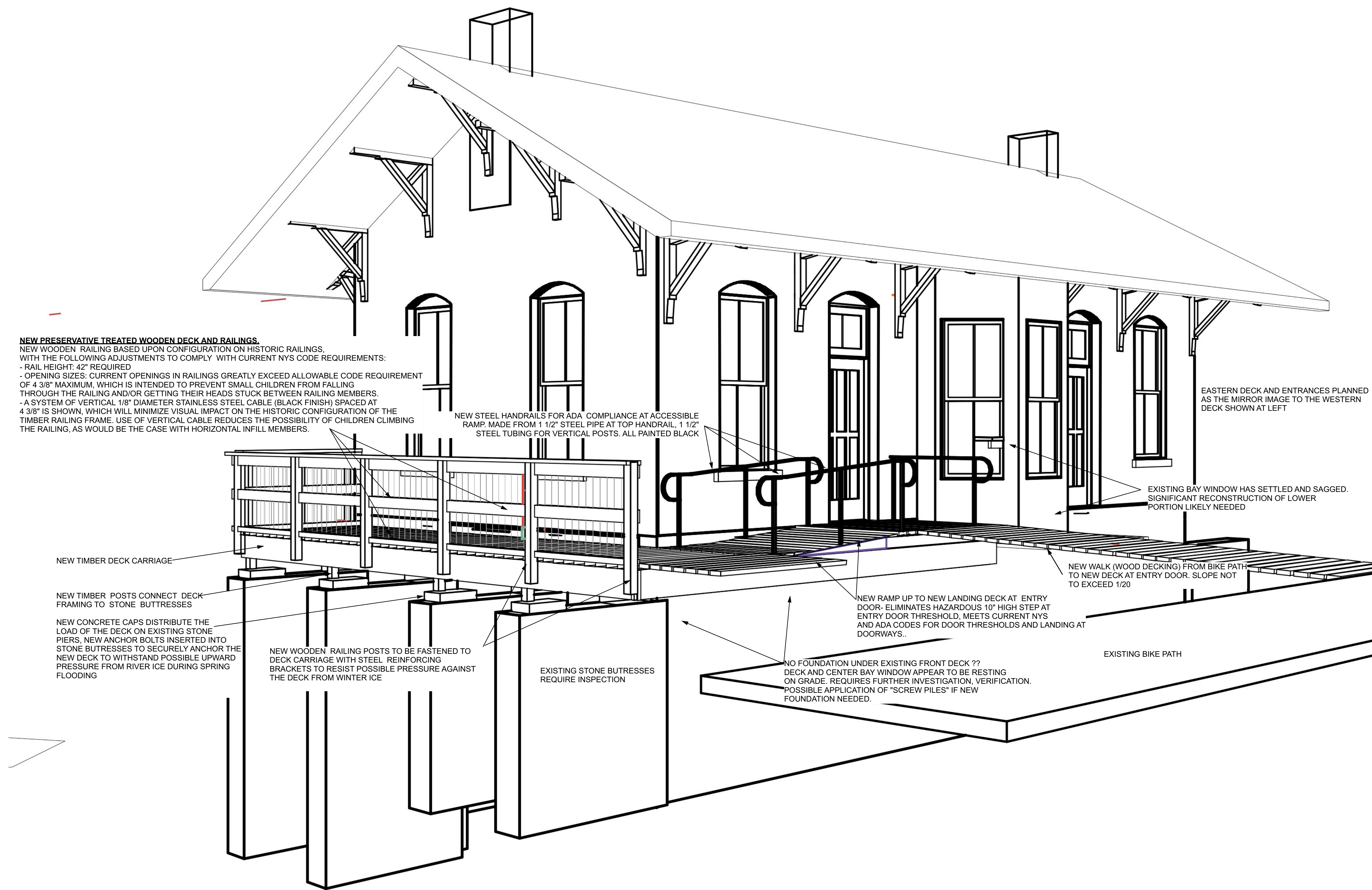
RAILING ALTERNATE 2- CONTEMPORARY PIPE RAILING (NEW ADDITION) AT SOUTH FACADE / ENTRY
