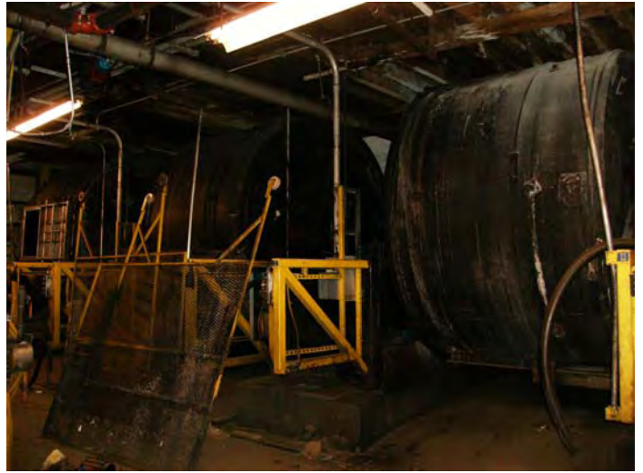
View of the former wooden mixing drums observed in the coloring area.
